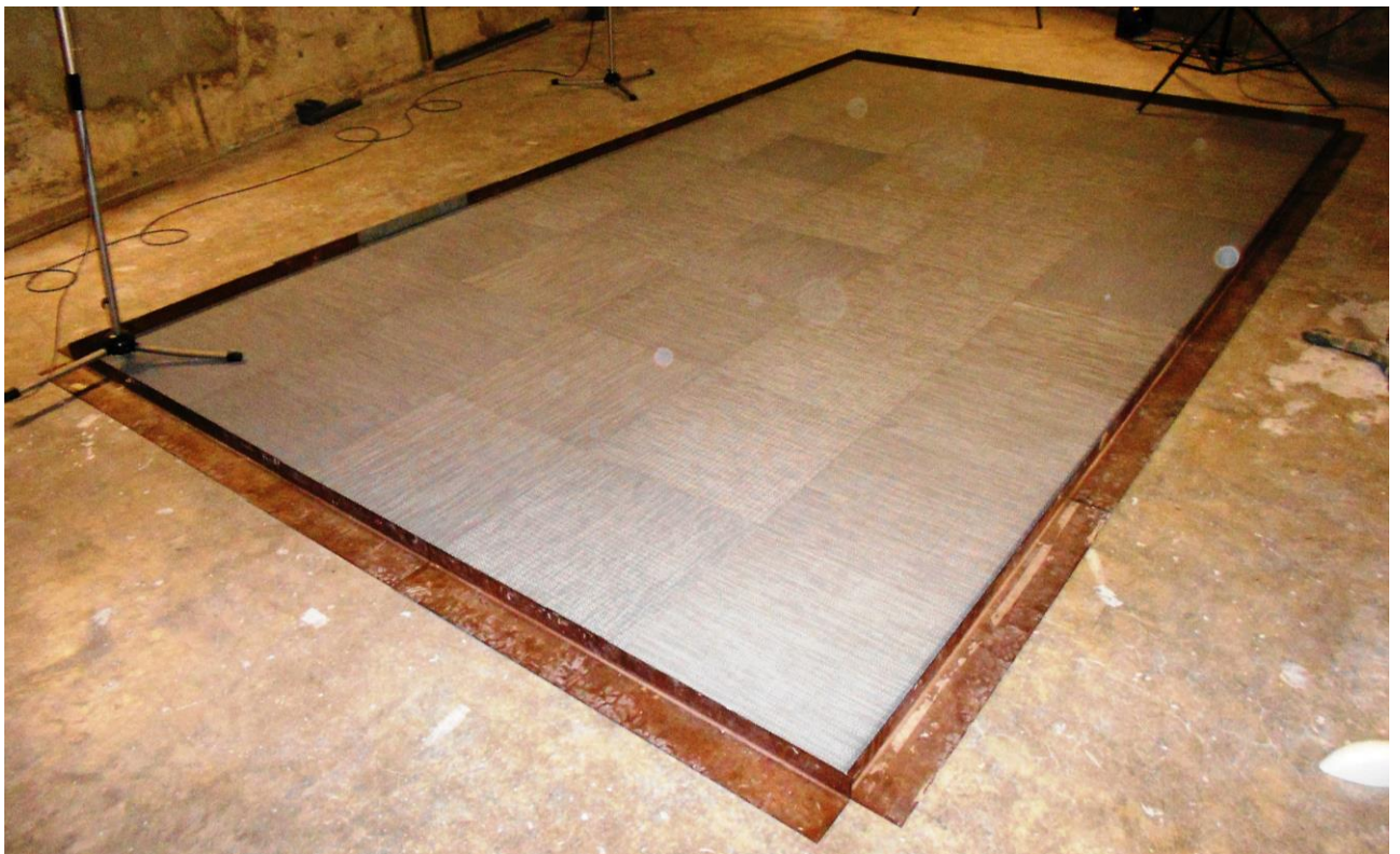
Figure 4: The Andrews Group Bolon Botanic Collection Woven Vinyl Flooring (500mm x 500mm tiles, 3.8kg/m 2 , 2.9mm thick) installed into the Reverberation Chamber for testing.
