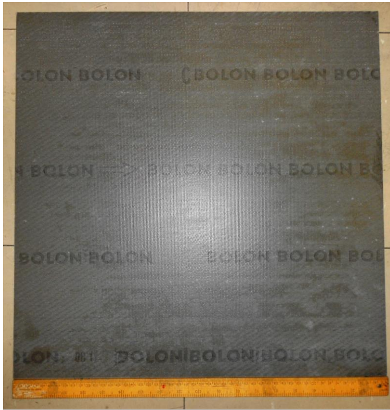
Figure 4: The Andrews Group Bolon Botanic Collection Woven Vinyl Flooring (500mm x 500mm tiles, 3.8kg/m 2 , 2.9mm thick) installed into the Reverberation Chamber for testing.
